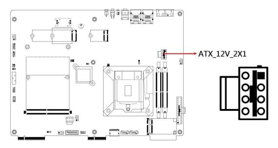
\* This connector supplies the CPU operating voltage.
